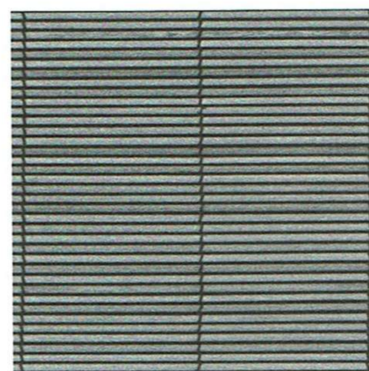
Details of a su with fine bamboo splints (top), a su with medium bamboo splints covered with a sha (middle), and a su made from kaya (bottom).
