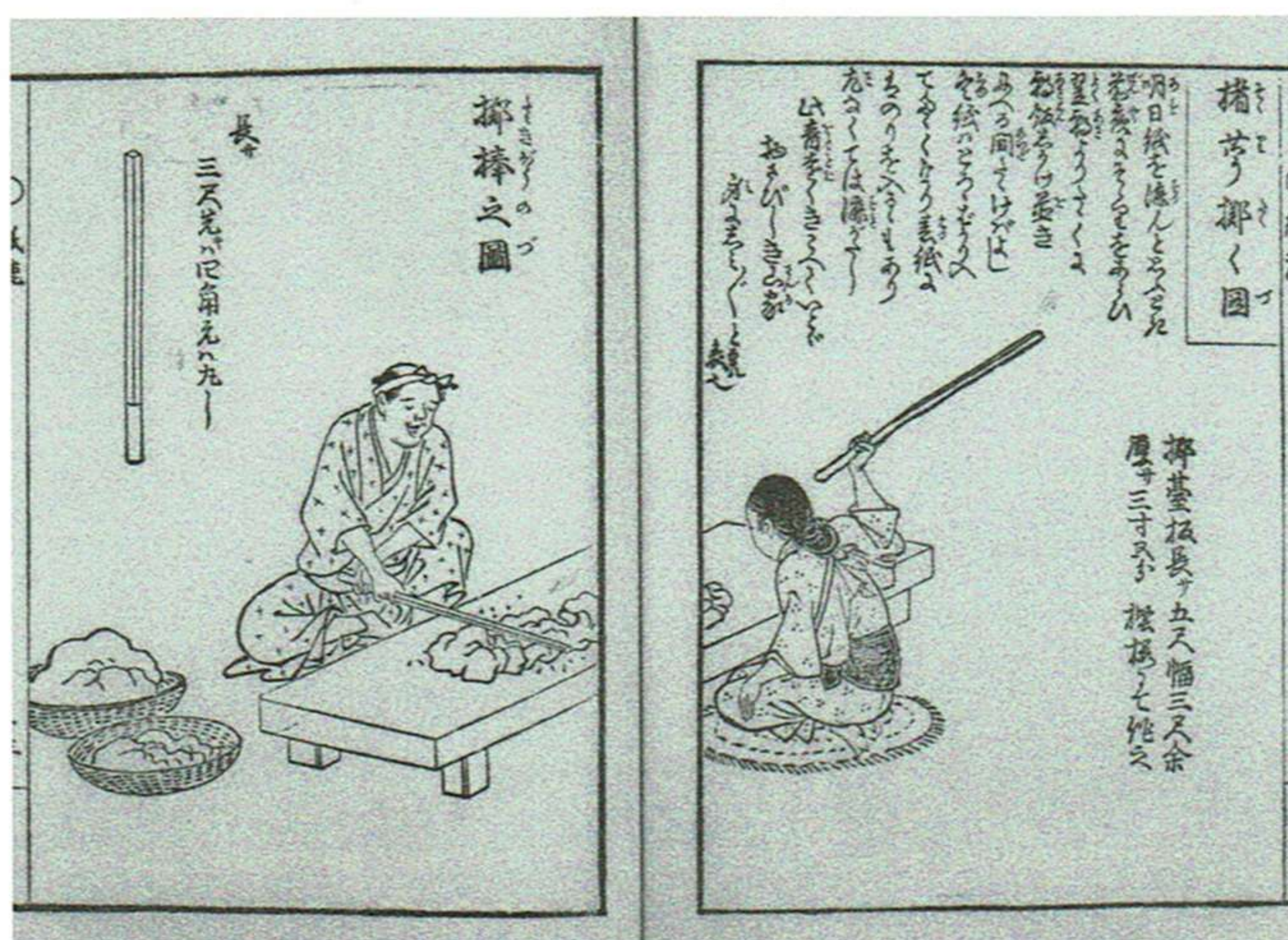
Two-page spread showing the beating step in the papermaking process, from Kamisuki Chohoki [A Handy Guide to Papermaking], originally published in 1798. All photos by and courtesy of the author unless otherwise noted.
