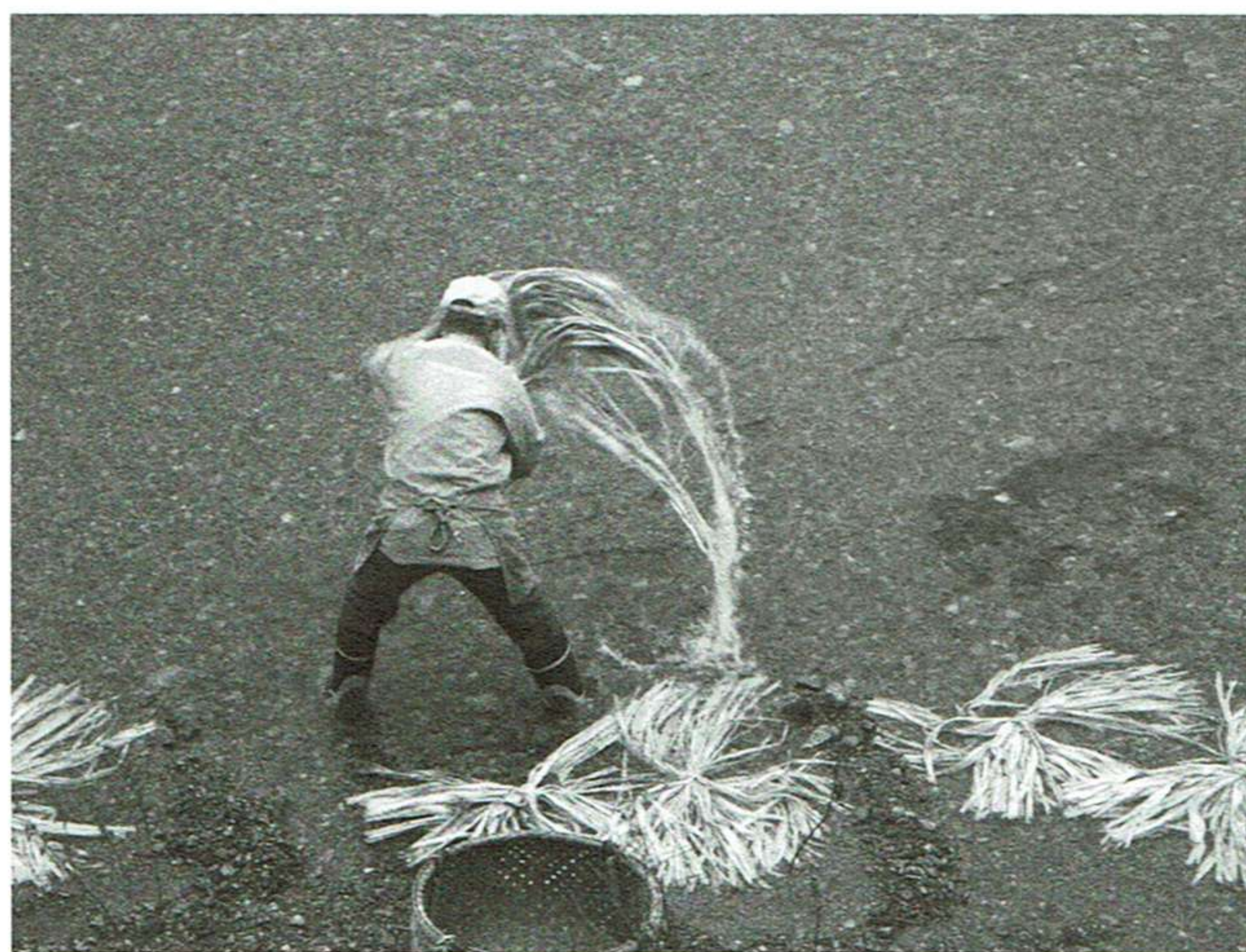
Fukunishi Hiroyuki rinsing kozo in the Yoshino river in preparation for kawazarashi (river-bleaching), a process which whitens the fiber by exposing it to the sun and the rinsing power of the river. 2006. Photo by and courtesy of Mina Takahashi.
